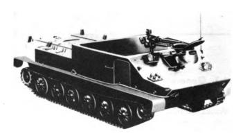
Figure 6-1. BTR-50P series tracked APCs. The original BTR-50P (above) has an open top. The newer BTR-50PK (below), with overhead armor covering, is in more general use. Most tank divisions use tracked APCs, either the newer BMP or BTR-50P types.
